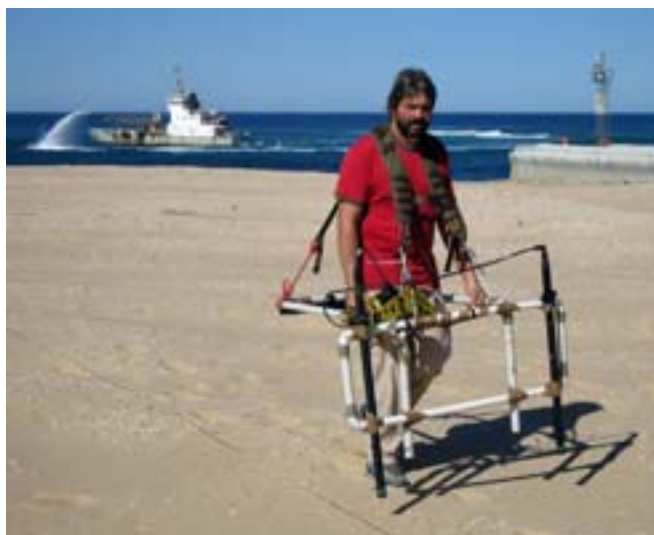
Figure 5: The sidcasting dredge April Hamer at work on the Lakes Entrance bar while Dr Bader conducts the gradiometer survey in grid E1 (photo: G. Hewitt)
